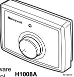
is designed to automatically adjust the humidity level based on indoor temperature and humidity, inferred or measured outdoor temperature, and the setting of the frost factor dial. The frost factor allows for variations in furnace size, window insulation and average daily climate temperature.
